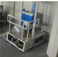
*Our mixing pump system is engineered to make sure that you will get the best possible mortar during printing. With our custom made rotor stator and additive pump we can easily adjust the printing material. An automatic startup kit, heating- and cooling unit are available as additional options.*
